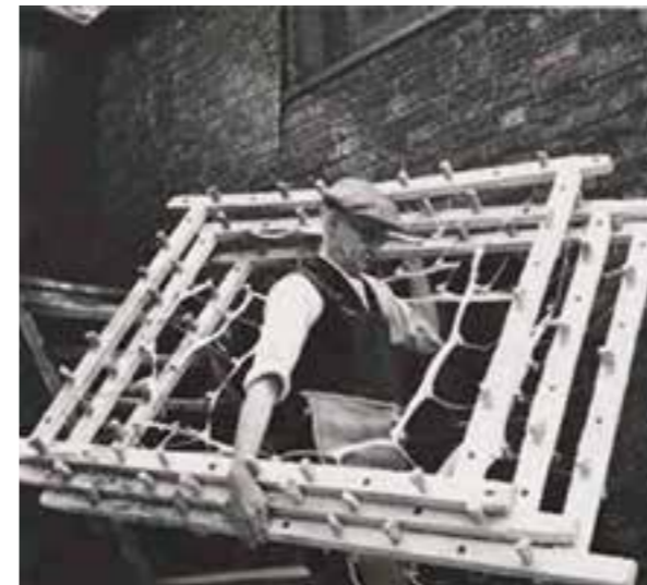
The racks used to stretch & cure the skins for transformation into Vellum.
